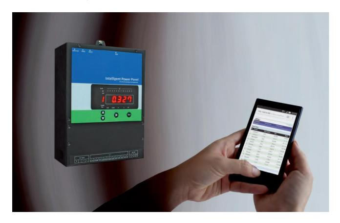
IPP series is a single/three phase remotely monitored power meter, built-in 12 independent measurement modules. User may select any one phase of the input voltage as a measurement reference. It supports the monitoring of twelve loops of 1P2W, or four loops of 3P3W/3P4W, or a hybrid combination, providing flexible application.
