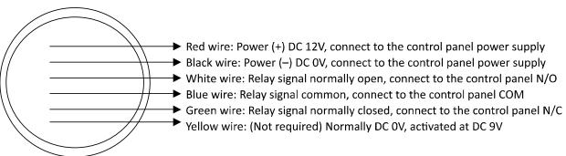
Note: Connect to either the control panel N/O or N/C terminal—only one is required.
